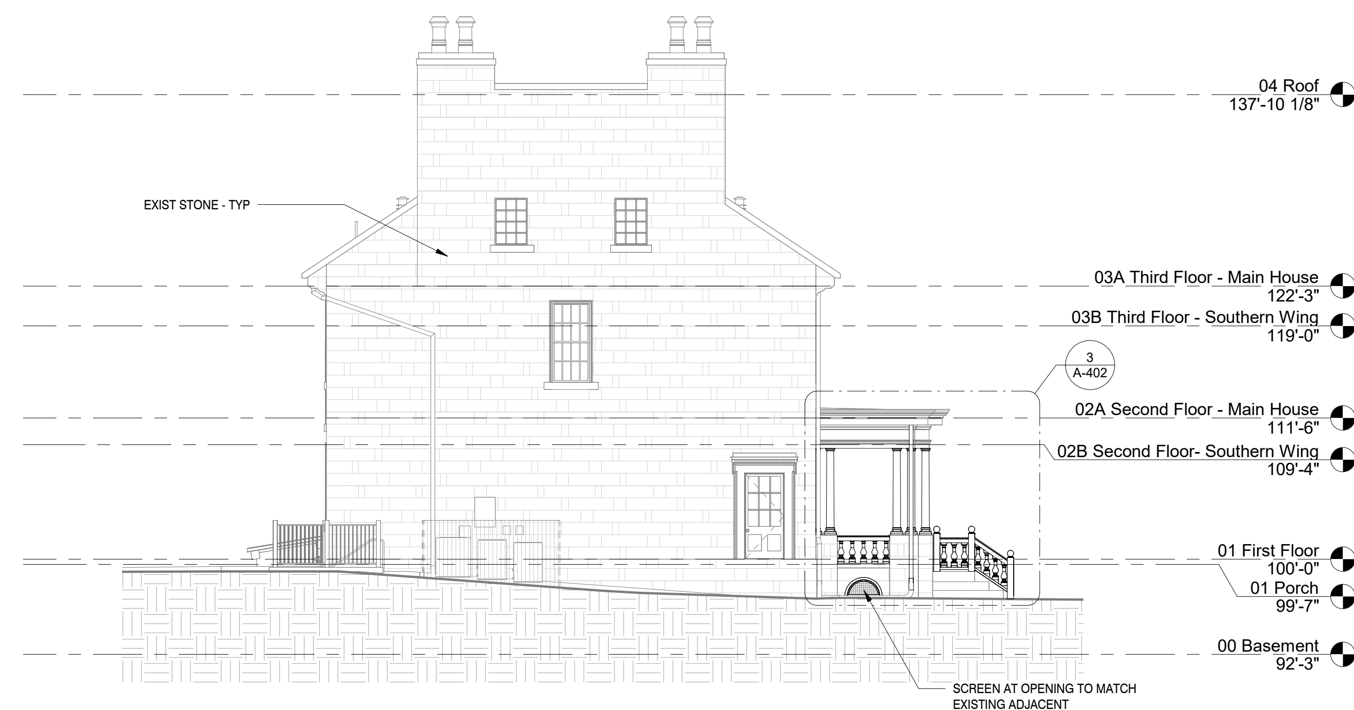
NORTH ELEVATION | 3 1/8" = 1'-0" | A-201
