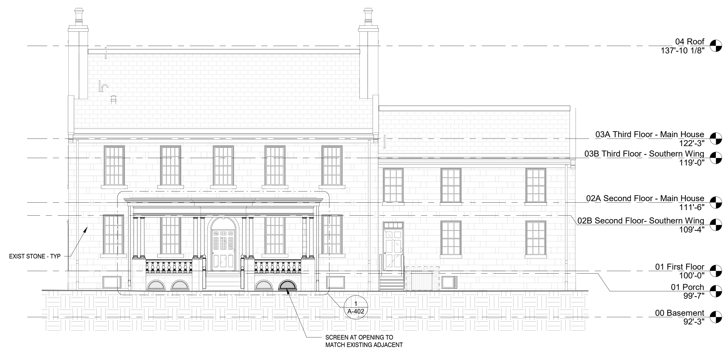
WEST ELEVATION | 1 1/8" = 1'-0" | A-201
